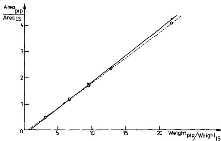
Fig. 4. Calibration graphs of peak surface area ratios versus weight ratios for piperine determination via micro-LC (○) and conventional LC (●). Internal standard, anthraquinone.
