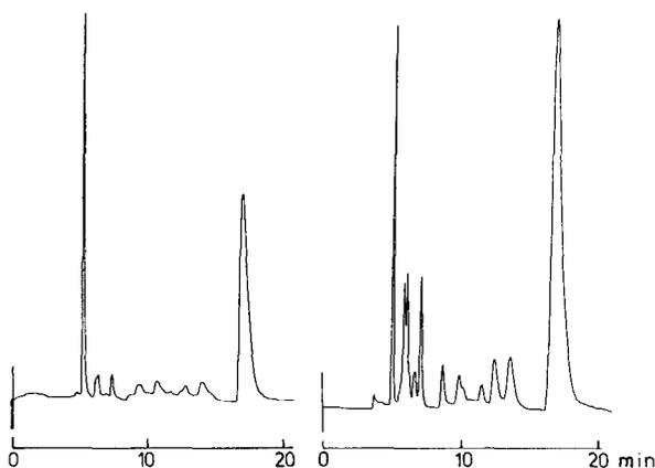
Fig. 5. Micro-LC traces for white Liebig pepper (left) and a Lampong pepper extract (right) with anthraquinone (first peak) as internal standard. Other conditions as in Fig. 2. The last peak is piperine.
