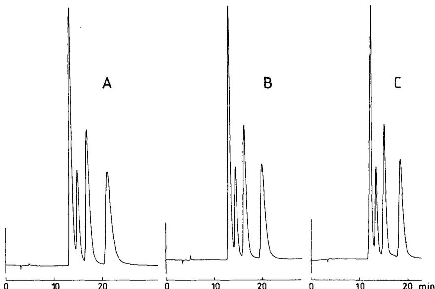
Fig. 3. Chromatograms obtained with a  $25 \times 0.46$  cm I.D. column packed with  $10\text{-}\mu\text{m}$  Polyphenol-RSiL. Mobile phase, hexane-THF (60:40) at 0.8 ml/min. UV detection at 252 nm. - Peaks in order of appearance: 1, chavicine; 2, isopiperine; 3, isochavicine; 4, piperine. Temperature: (A)  $30^\circ\text{C}$ ; (B)  $40^\circ\text{C}$ ; (C)  $50^\circ\text{C}$ . Back-pressures: (A) 34; (B) 32; (C) 30 bar. Sample injected:  $10\ \mu\text{l}$  of the same solution as in Fig. 2.
